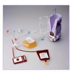
3 Remove most red blood cells and plasma and isolate stem cells into 20 ml using the AutoXpress device and add 5 ml cryoprotectant
