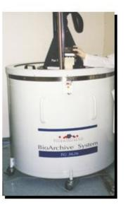
Initiate automatic Controlled Rate Freezing and archival of NCBP unit in BioArchive System
